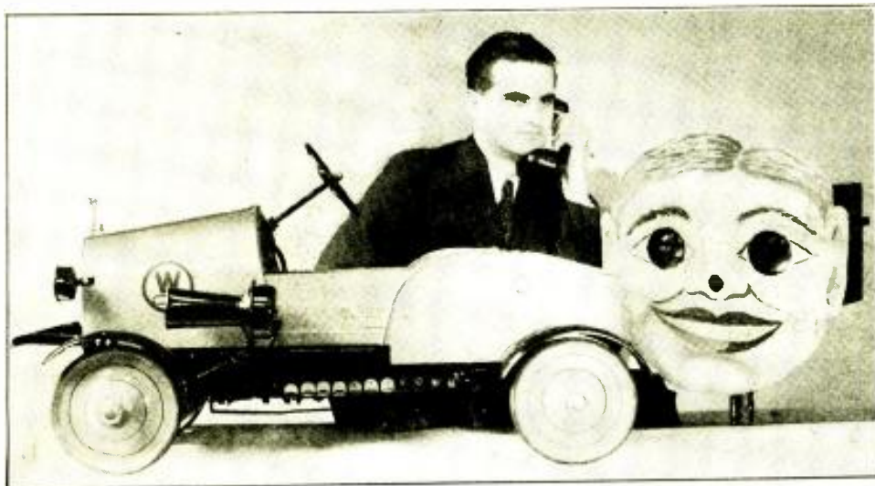
The apparatus used in the control of an automobile by word of mouth, at the Radio World's Fair of 1930. The signals were in this case given by light at short-range, instead of radio, but the principle is similar. (Photo by Westinghouse Elect. & Mfg. Co.)
